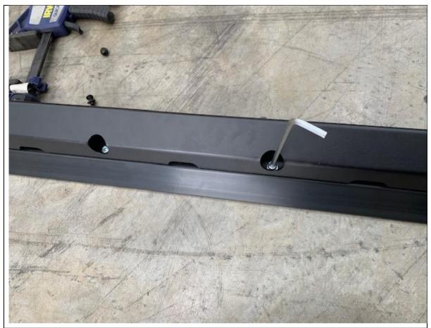
25. Thread cap screws into each hole.
