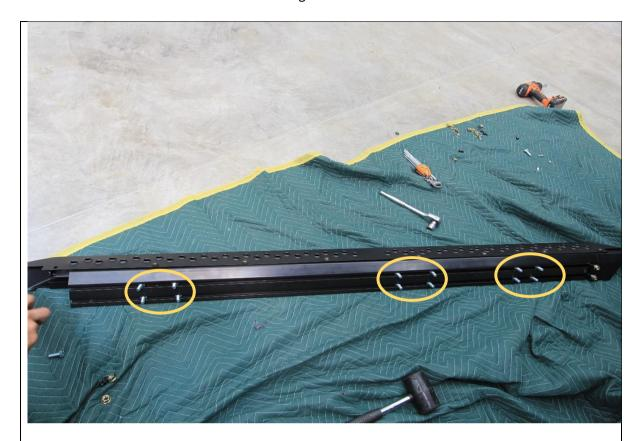
33. Slide the 12x M10x25 Hex bolts into the T slots on back side of extrusion. 6 bolts per slot.
