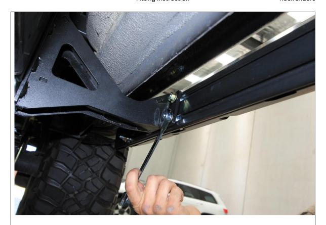
46. Tighten all mount to slider M10 flange nuts using 15mm spanner. A ratcheting spanner makes this process easier.
