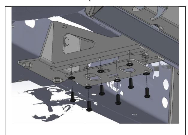
47. Once front mount bolts are tightened, fit the brace plate using 6x M8x20 Button Head, M8 Flat washers and M8 Flange Nuts.
